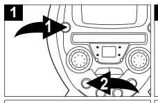
Press the POWER button 1 to turn the unit on. Rotate the MONITOR switch 2 to the CD position.
